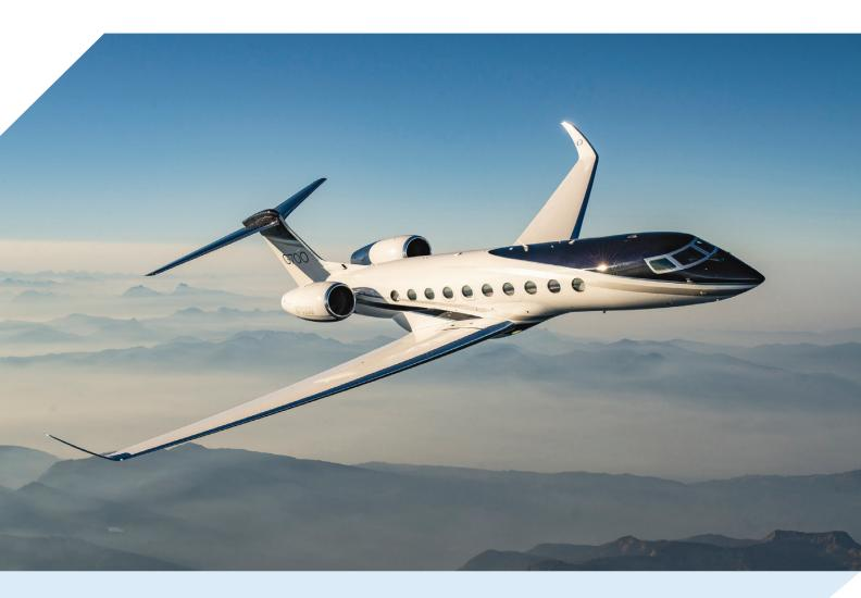
The ultra-long-range, ultra-large-cabin G700 combines our most spacious cabin with our advanced Symmetry Flight Deck, the most technologically advanced in the industry. The aircraft has a maximum range of 7,750 nautical miles and is capable of speeds up to Mach 0.935.
